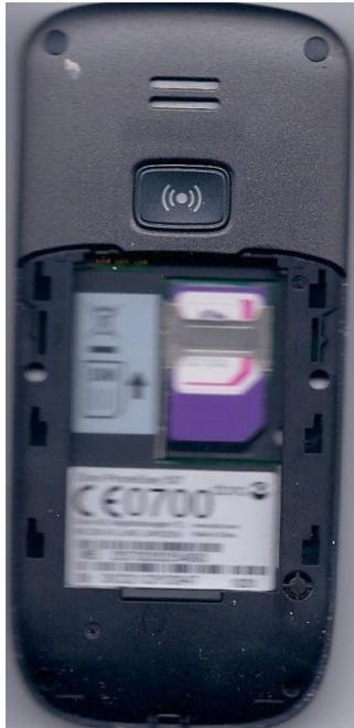
You must sign a subscription with any supplier. This means you get a SIM-card, a pincode and a pukcode. SIM-card will be installed in phone. Do this by pulling backpart down, take away battery and pull SIM-card up.
